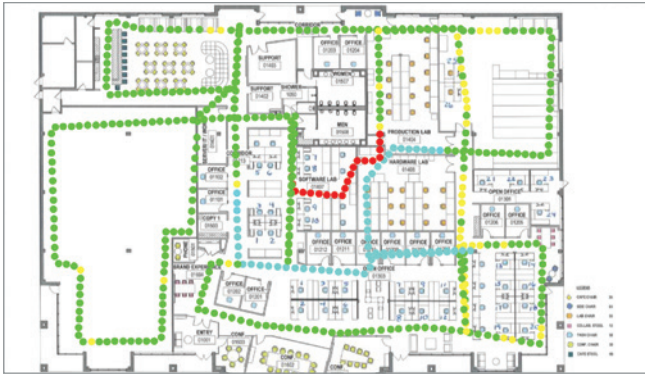
▲ Walk Testing Supports automated uplink testing with SeeHawk Monitor system
